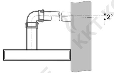
**Fig. 3:** inclination angle of the exhaust air pipeline
