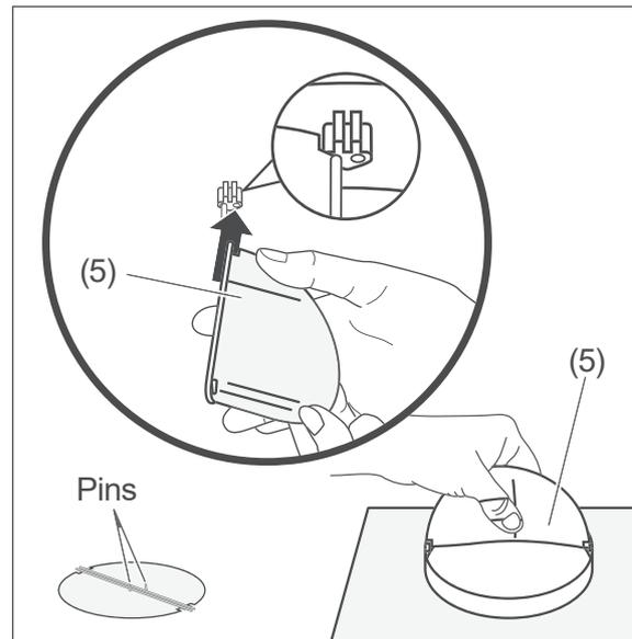
1. Place the two halves of the check valve (5) into the opening on the top of the Exhaust hood(1).
