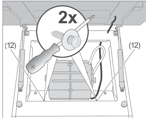
8. Turn two round-head screws (12) into the prepared wall plugs to secure the Exhaust hood, and screw the Exhaust hood tightly to the wall.
