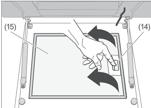
5. Open the locks (14) on the grease filters (15) and carefully pull the grease filters downwards to remove them.
