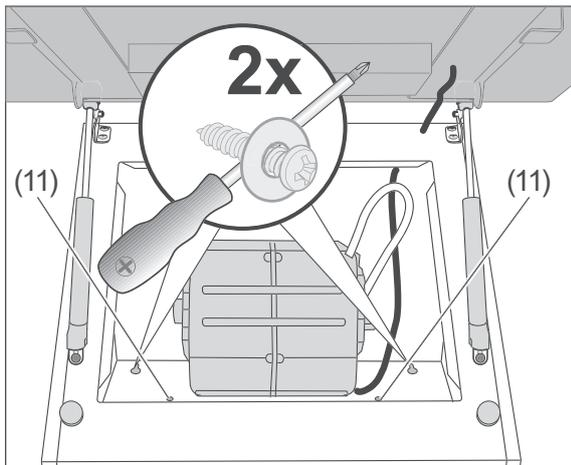
6. Carefully hang the Exhaust hood on the two round-head screws (11) using the key-hole openings.
