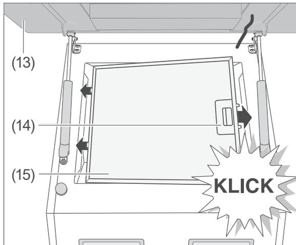
5. Once the grease filter (15) is fully dry, insert it with the pins into the openings.
