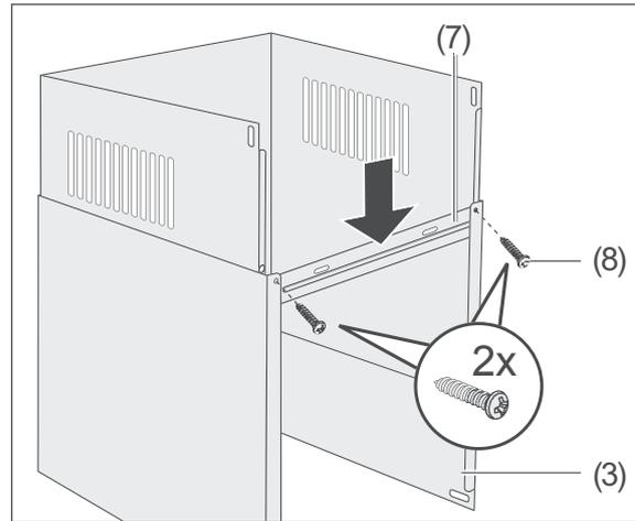
5. Place the retaining plate (7) onto the lower flue screen (3) so that it lines up with the chamfers on the inside. (Screws and elongated holes should point upwards).
