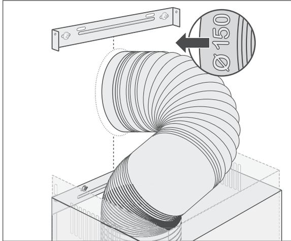
9. Only for exhaust air operation: Insert the exhaust air hose (4) into the connection at the wall break (hose end with 150 mm diameter).
