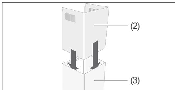
4. Push the upper part (2) of the flue screen halfway into the lower part (3) of the flue screen.
