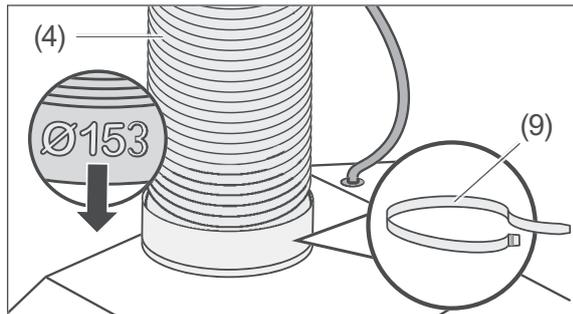
1. Insert the end of the exhaust air hose (4) with the larger diameter (153 mm) into the connection with the check valve.
