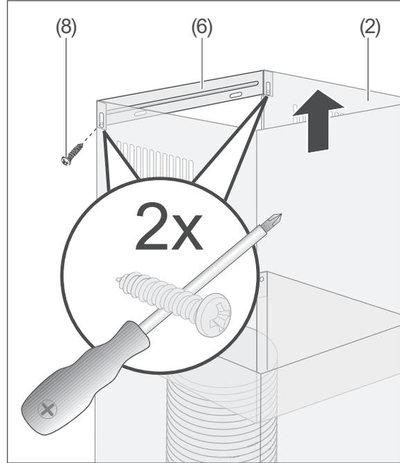
11. Pull the upper part of the flue screen (2) all the way up to the wall bracket for the upper flue screen (6).
