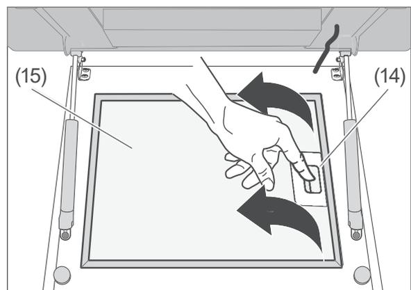
3. Open the locks (14) on the grease filter (15) and carefully pull it downwards to remove.
