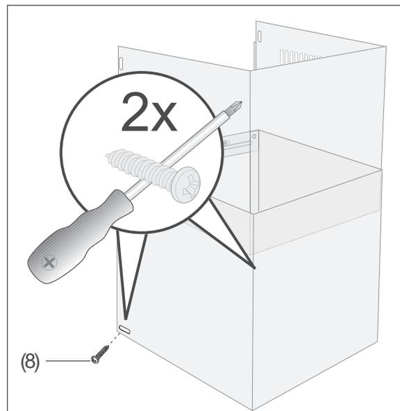
8. Screw the lower part (3) of the flue screen with 2 plate screws (8) to the sides of the exhaust hood (1).
