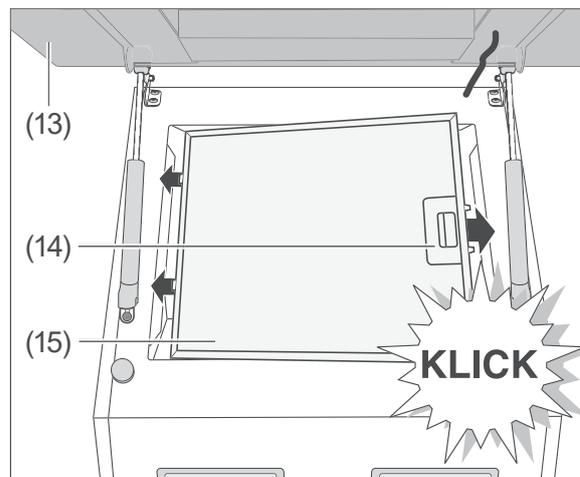
9. Place the grease filter (15) with the pins into the openings.
