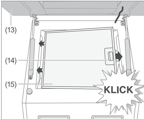
6. Place the grease filter (15) with the pins into the openings.
