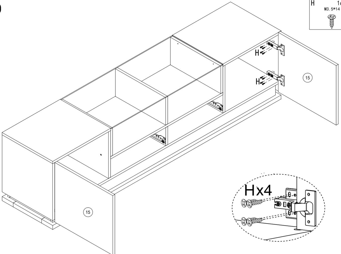
When the hinges are installed, you can refer to the pictures to adjust crevice of the doors till it's perfect:
