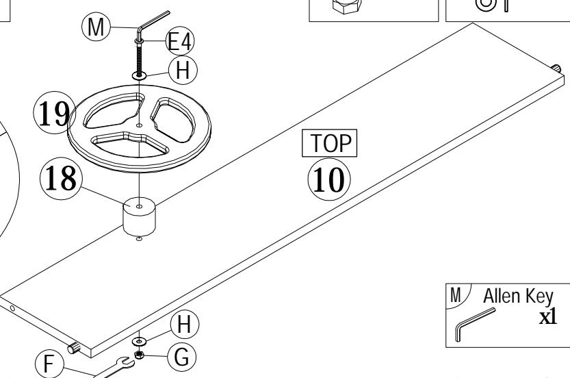
Using the Spanner (F) and Allen Key (M), ensure that the Bolt (E4) and Locking Nut (G) are securely fixed and that the wheel can still turn freely.
