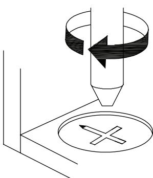
**EN**\_ Turn cam lock clockwise to tighten.
