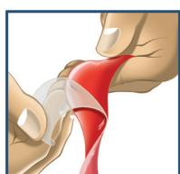
2. Remove the transparent film from the upper side of the tape and place the tape on the element to be repaired.
