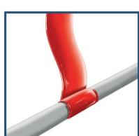
3. Apply the tape and hold it in place with your thumb. Pull the tape tight and wrap it around one time completely with complete overlap (tape is fixed in position for further wrapping).
