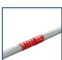
5. For the final winding, pull less tightly on the tape and make sure that it overlaps itself completely. Press on the tape for 10 seconds until it is fixed in place.
