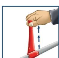
4. Overstretch the tape consistently by about 200% and wrap it around in an overlapping manner while pulling on it tightly. When doing so, make sure that the tape overlaps itself with at least 50% of its width (self-fusing).
