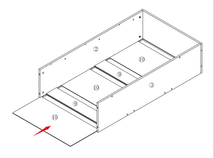
STEP 1: Insert No. 9 and No. 10 plates into the notches of No. 2 and No. 3 plates in sequence.
