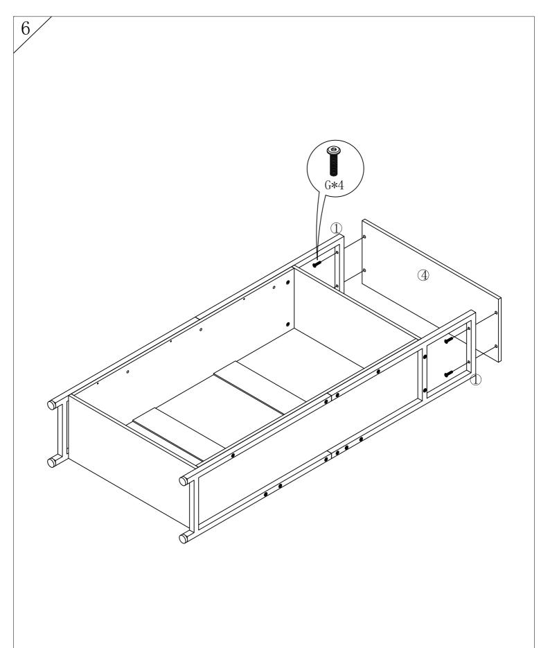
STEP 1: Connect and fix the G screw through No. 1 steel frame and No. 4 plate.
