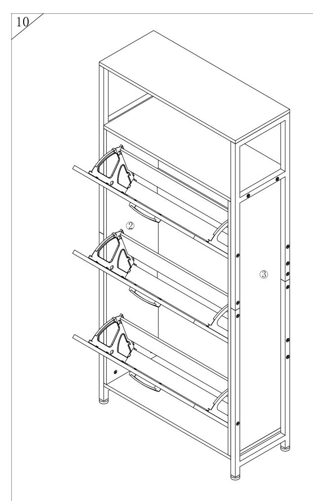
STEP 1: Insert the whole part installed in step 9 between plate 2 and plate 3.
