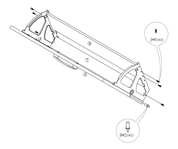
STEP 1: Fix j-screw through A-part to 7-plate and 8-plate, STEP 2: Insert the H fitting into the hole corresponding to the side of plate 6.
