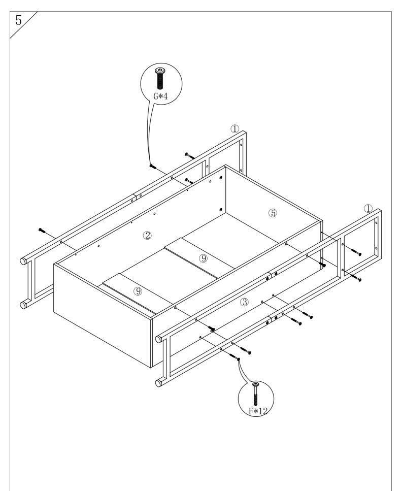
STEP 1: Connect and fix F screw through No. 1 steel frame to No. 5 and No. 9 plate. STEP 2: Connect and fix the G screw through No. 1 steel frame to No. 2 and No. 3 plates.
