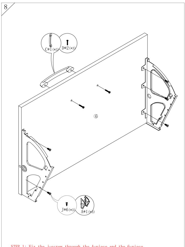
STEP 1: Fix the j-screw through the A-piece and the 6-piece. STEP 2: Fix Screw D through plate 6 and handle C.
