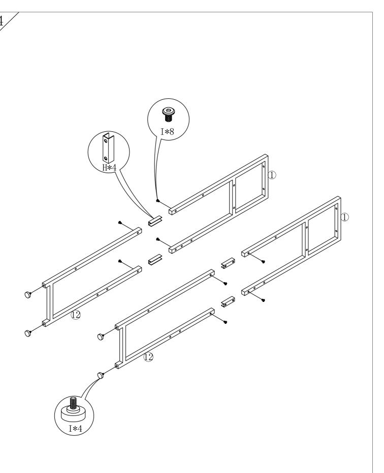
STEP 1: First, insert the H fitting into the No. 1 and No. 12 steel frames, then use the I screw to connect and fix the H fitting through the No. 1 and No. 12 steel frames,
