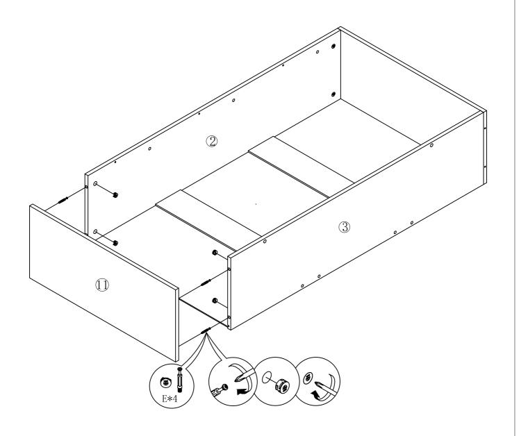
STEP 1: first the e-eccentric rod screw into 11 plate, STEP 2: then the E-eccentric wheel into 2,3 plate and lock.
