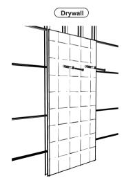
▲ If the cabinet does not fit the wall after the hanger is installed, adjust the two cross screws on the back of the hanger. please refer to last page details.
