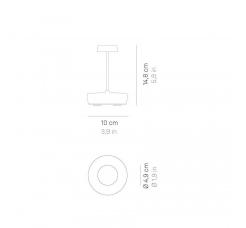
Swap mini is a battery-operated, portable and rechargeable table lamp. It has a contact charging base and dimmer touch control. Thanks to its small size (height 14.8 cm and diameter 10 cm) it creates the right atmosphere both indoor and outdoor.
