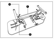
Use parts K and N to install the two crossbars of part F.
