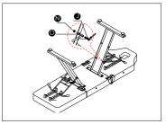
Use parts J, N and O to install the two adjustment handles of part E.
