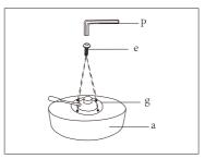
Install the base with 4 pieces mechanism screws(e).
