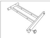
Check all the part list after box opened.Install part G on the foot.
