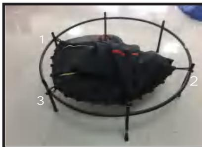
11 Next, count back around the jump mat 8 loops and repeat steps 1-3 attaching the 3rd cord about half way between the 1st & 2nd cords.
