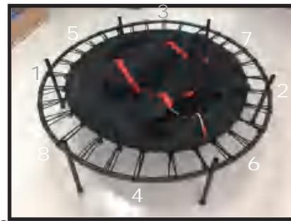
12 Then, from the 3rd attached cord, count around the jump mat 16 loops and repeat steps 1-3 to attach the 4th cord. Numbers on the picture above show the approximate positions of the first 8 suspension cords. Continue connecting the remaining cords as shown in steps 1-3, but always connect a cord, and then switch to the opposite side of the trampoline to connect the next cord. Attaching the cords in this manner is important, as it will ensure even-tension around the entire jump mat.
