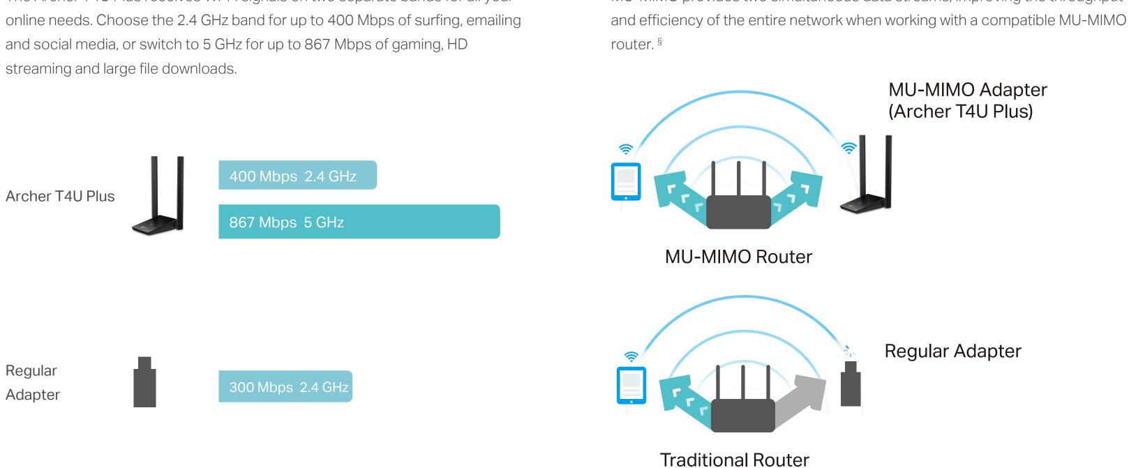
MU-MIMO provides two simultaneous data streams, improving the throughput
