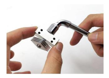
3.2 Lie the hotend assembly on a flat surface, rotating the heat sink so that the fixing screw is facing outwards
