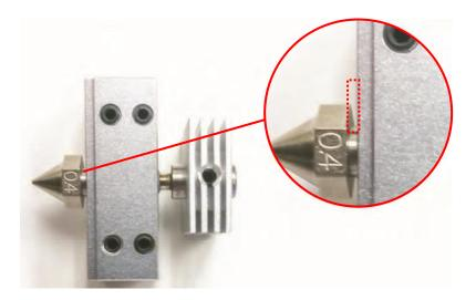
STEP 2: Tighten the Throat Tube
