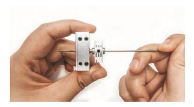
1.3 Screw the new nozzle into the heating block. Do not tighten completely. Ensure that there is a visible gap between the nozzle and the heating block.
