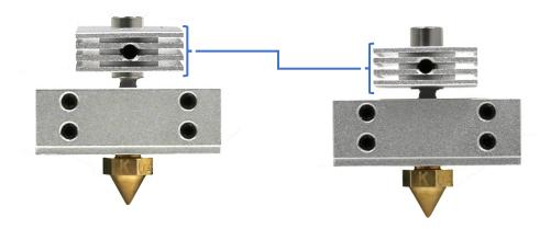
3.4 If you do not have a silicone sock, adjust the heat sink so that it is flush with the bottom of the large cylinder.
