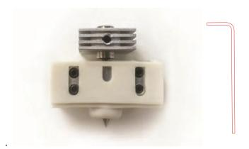
3.3 Move the heat sink down so that it rests on the silicone sock, and tighten into place.
