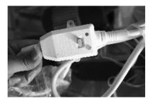
The creepage protector will automatically cut off the circuit if the current is too high.
