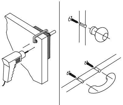
**FIXING THE HANDLES OR KNOBS**
