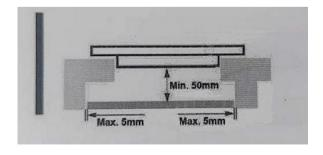
There are ventilation holes around outside of the hob. YOU MUST ensure these holes are not blocked by the worktop when you put the hob into position. Be aware that the glue that join the plastic or wooden material to the furniture, has to resist to temperature not below  $150\,^{\circ}\mathrm{C}$ , to avoid the unstuck of the paneling. The rear wall, adjacent and surrounding surfaces must therefore be able to withstand an temperature of  $90\,^{\circ}\mathrm{C}$ .
