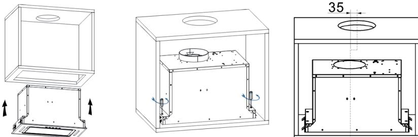
Slide the cooker hood into the cabinet housing. Tighten the screws from the top. Note for the outlet hole in the cabinet: The air outlet at the top of the cooker hood is offset by 35 mm, measured from the centre of the hood.
