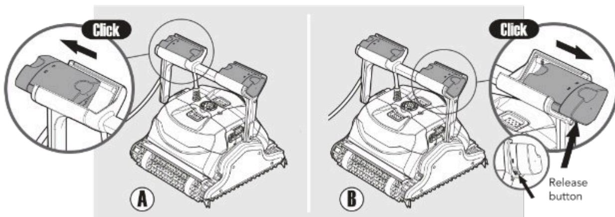
To move the floats back to their original position: while pressing the release button on the base of the handle float – push the handle float back.
