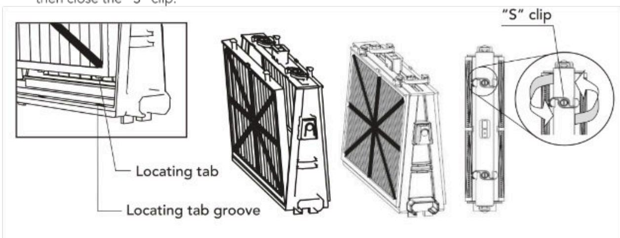
Reinstall the base frames with filters according to the diagram.
