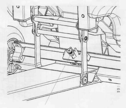
Steering nut: screwing the nut clockwise (use enclosed 10 mm wrench), you make steering harder; By rotating the nut anticlockwise, you make it softer NOTE: ROTATE NUT, NOT BOLT!
