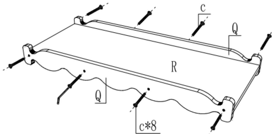
Connect the 2 slide side panels Q to the slide R and fix it with 8 pieces of M6\*35. Set aside for later use after installation.
