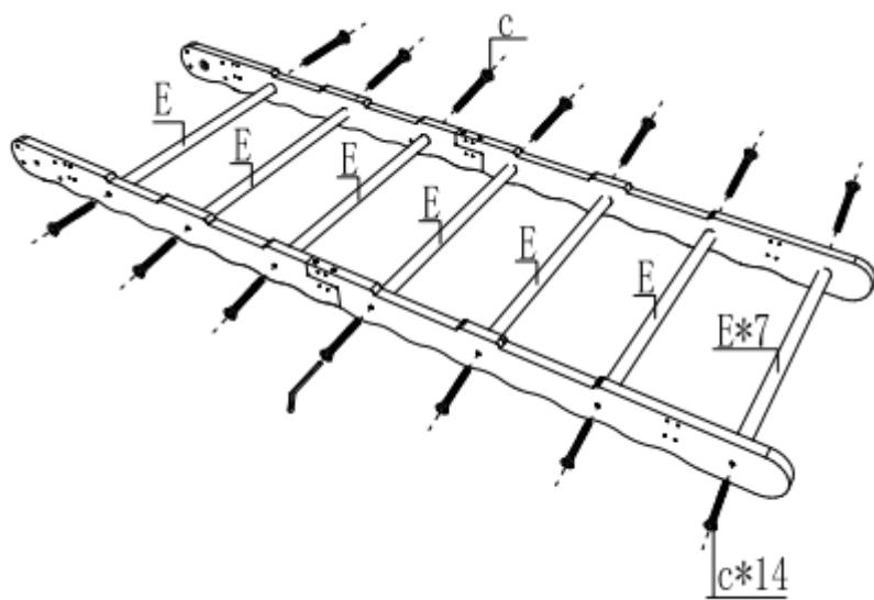
Insert 7 pieces of E round sticks into the corresponding round holes and fix them with 14 pieces of M6\*35 screws. Set aside for later use after installation.
