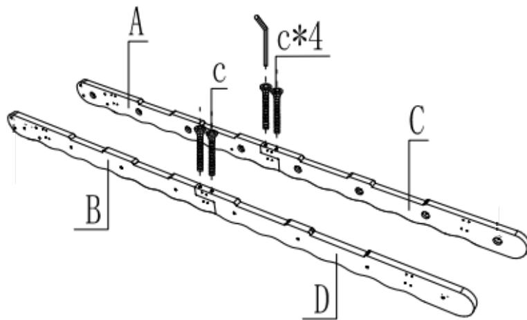
Connect A and C, B and D correspondingly together, and fix it with 4 pieces of M6\*35 screws.
