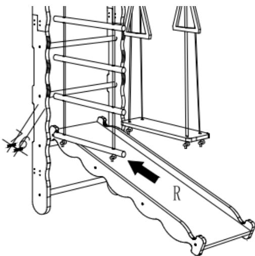
Place the slide on the first or second round stick of the main body, and the whole installation procedure is complete (**please do not place it on the third or upper round stick, otherwise it will cause danger due to the excessive inclination angle**)
