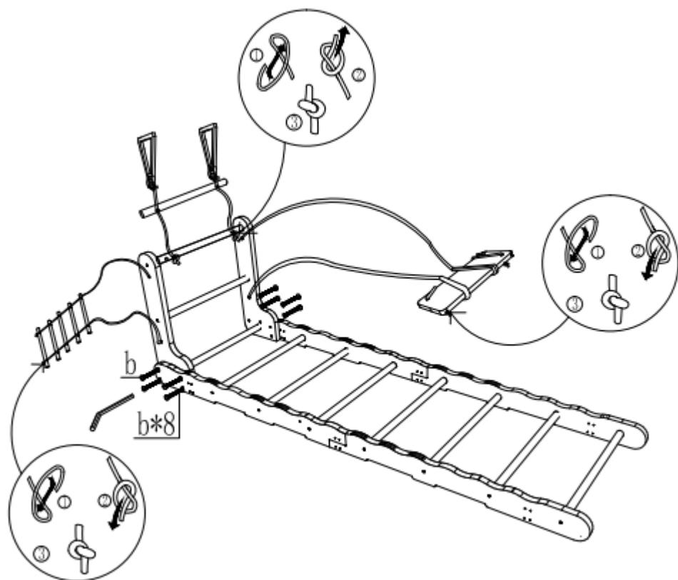
Connect the parts installed in the second and third steps with 8 pieces of M6\*50. Set aside for later use after installation.
