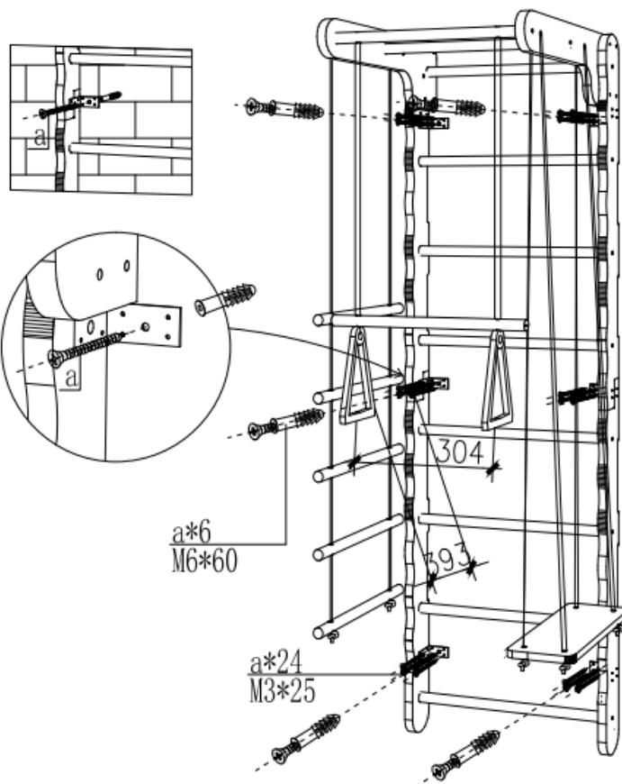
First, open six small holes on the wall suitable for M6\*60 screws according to the position of the center round hole of the six wall-hanging iron pieces of the climbing frame. Second, put the M6\*60 into the holes, tighten it. and then unscrew the nut, then align the wall-mounted iron piece of the climbing frame with the hole, insert the nut into the center hole of the iron piece and tighten. Finally, each iron piece is fixed again with 4 M3\*25 screws
