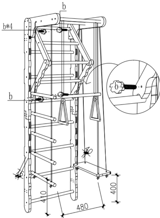
Use 4 pieces of M6\*30 screws to fix the part installed in the fourth step into the main frame.
