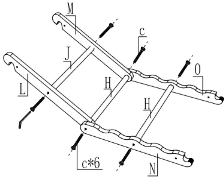
Insert 1 piece of round stick J into L and M and fix it with 2 M6\*35 screws, then Insert 1 piece of round stick H into L and M, at the same time, connect it with N and O, fixed with 2 pieces of M6\*35. Finally, insert a H into O and N and fix it with 2 pieces of M6\*35. Set aside for later use after installation.
