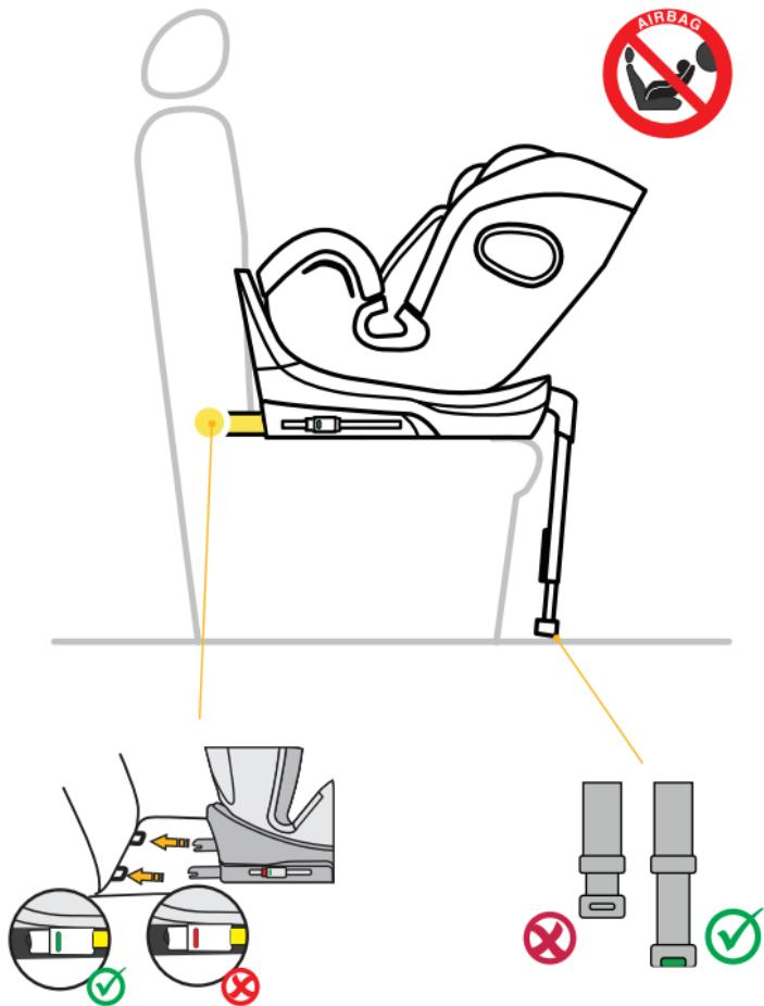
1. Set the child car seat to seat position 4 and rotate it so that it faces seat position R in a rear-facing orientation.
