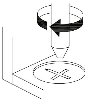
**EN**\_Turn cam lock clockwise to tighten.
