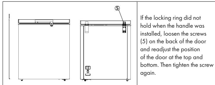
If the locking ring did not hold when the handle was installed, loosen the screws (5) on the back of the door and readjust the position of the door at the top and bottom. Then tighten the screw again.
