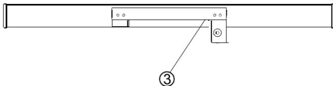
Press the handle cover (3) onto the handle until it clicks into place.
