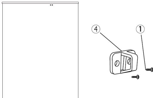
Then fasten the latch (4) to the freezer with screws.
