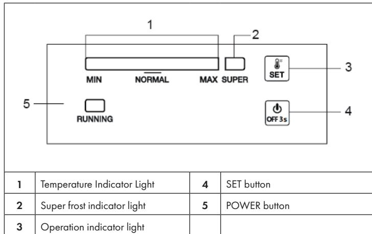
When you plug in the connector, all lights light up briefly. After that, the unit runs with the last settings made.
