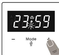
2. Select the desired time period using the “**+**” and “**-**” keys while “**4**” is flashing.
