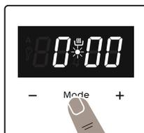
1. Press the "MODE" for 2 sec to deactivate keylock and the dot in the middle of the screen will start to flash.
