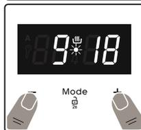
2. Adjust the time while the dot is flashing using the "+" and "-" keys.
