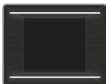
**Static Cooking Function:** The oven's thermostat and warning lights will switch on, and the lower and upper heating elements will start operating. The
