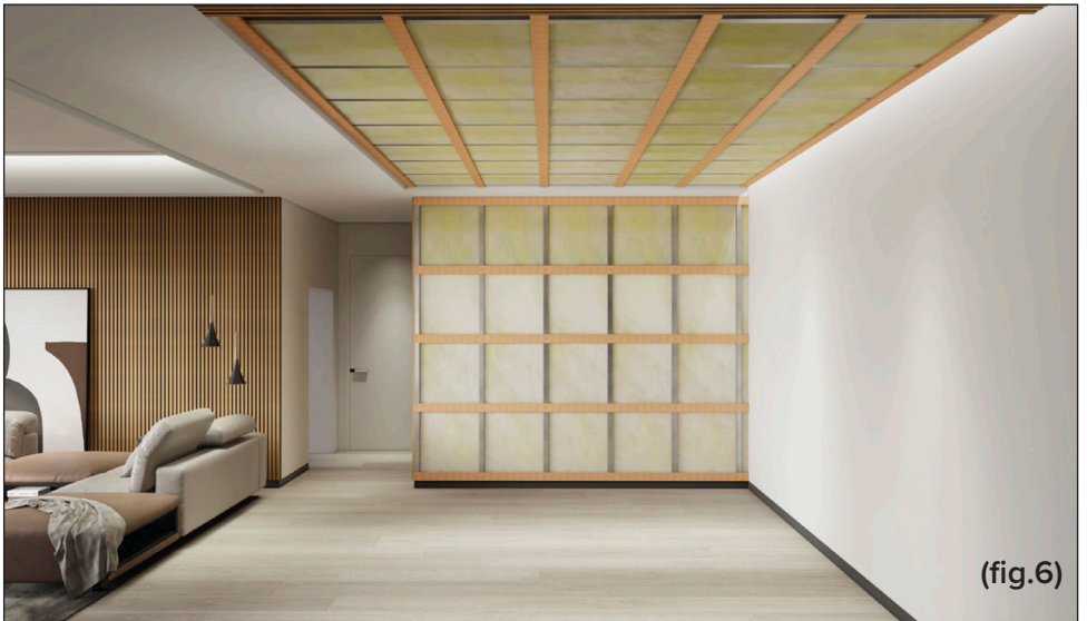
Insert the sound-absorbing wool between the studs and wooden battens (fig.6)
