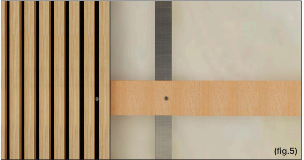
Mounting the slat panel with screws. (fig.5)
