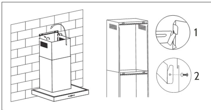
1. After drilled the 2 holes and fixed the hook, hang the chimney cover by matching the both side lock (Pic1).
