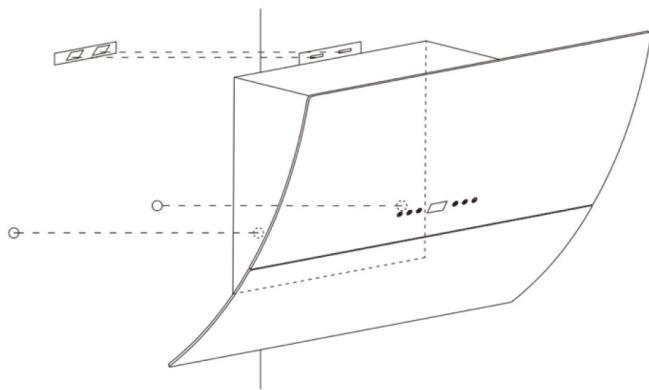
For inclined panel model, you need to drill 2 x 8 mm extra holes an use screw plugs and screws befor installation.
