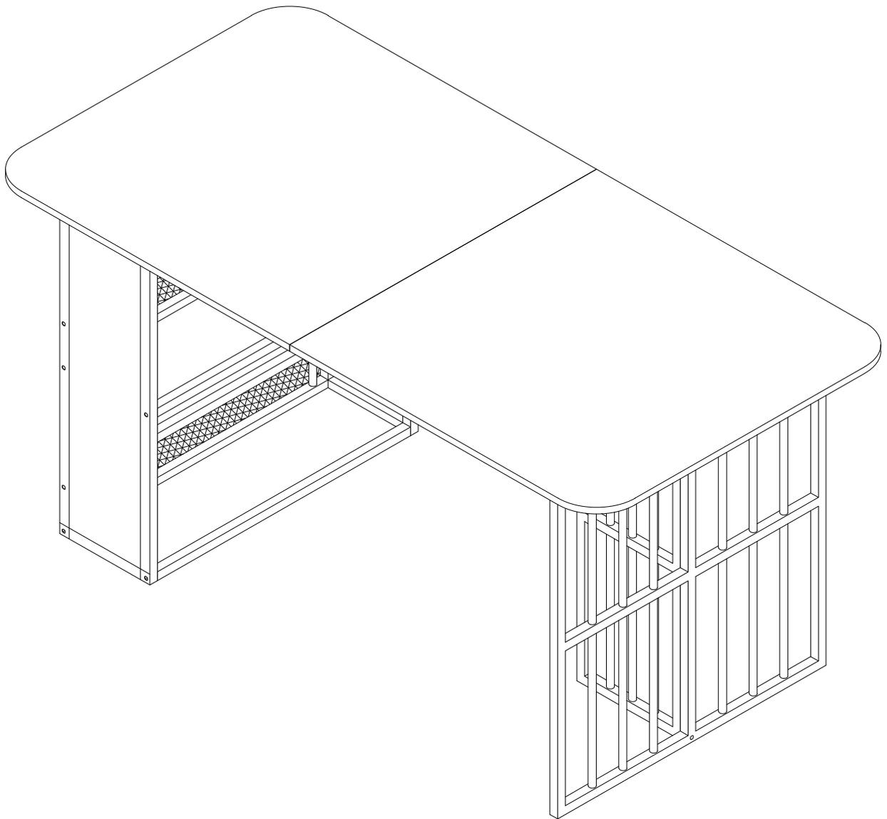
Attention:Don't tighten the screw before all screws are in place
