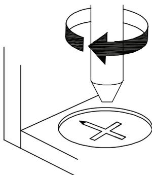
**EN\_**Turn cam lock clockwise to tighten.
