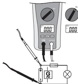
→ As soon as a minus "-" appears for the direct voltage in front of the measuring value, the measured voltage is negative (or the measuring tips have been mixed up).
