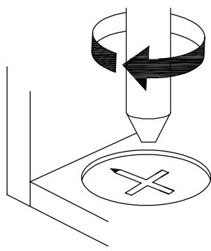
**EN** Turn cam lock clockwise to tighten.
