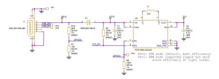
VBUS is the 5V input from the micro-USB port, which is fed through a Schottky diode to generate VSYS. The VBUS to VSYS diode (D1) adds flexibility by allowing power ORing of different supplies into VSYS.
