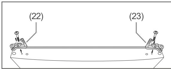
2. Loosen the screw on the plastic insert (22) of the appliance door (2) and remove the plastic insert.
