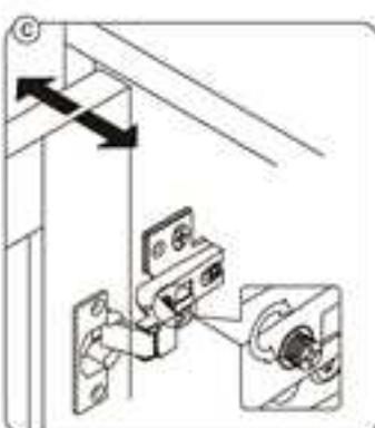
**EN** To adjust the door laterally adjust the screw as shown by turning clockwise or anti-clockwise.
