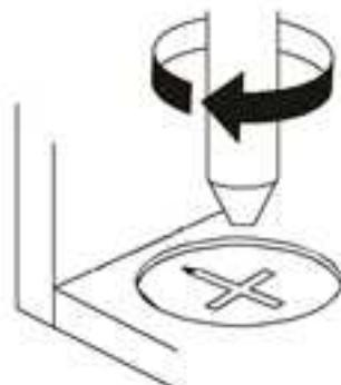
**EN**\_Turn cam lock clockwise to tighten.
