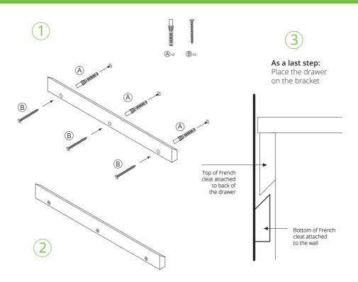
**Wall fixings:** Because of the variety of different wall types, Woodek cannot provide you with exact fixing you will need to fix this product to the wall. You must first identify the type of the wall you intend to fix product onto and then contact your local hardware store to get the appropriate fixings.
