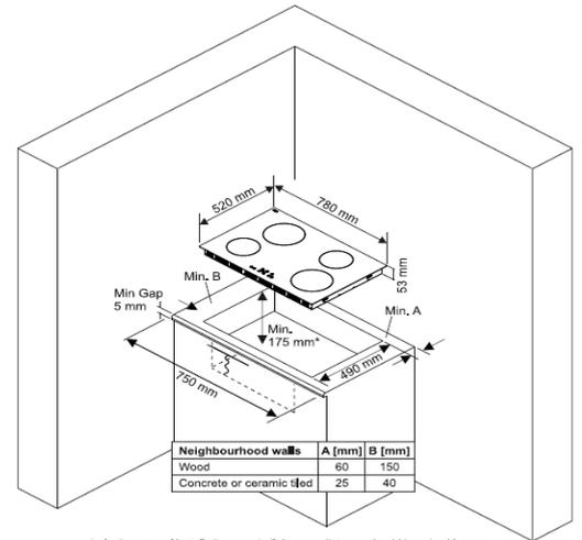
\*: In the case of installation over built in oven, distance should be min. 10 mm.
