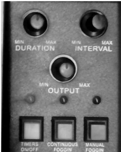
With the rotary controls of the remote control duration, interval and volume of the fog output can be adjusted. With OUTPUT controller set 0, there is no function.
