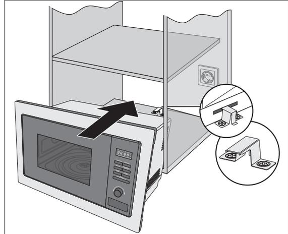
5. Push the appliance into the installation compartment until the front panel meets the frame of the installation compartment.
