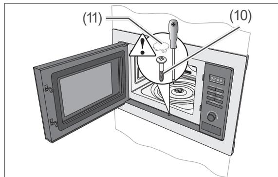
6. Secure the appliance against sliding out with the third screw (10).
