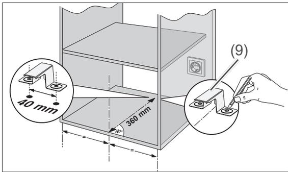
3. Position the anti-tip device (9) centrally at the end of the auxiliary line and mark the positions of the drill holes with a pencil. There must be a clearance of 40 mm between the drill holes.
