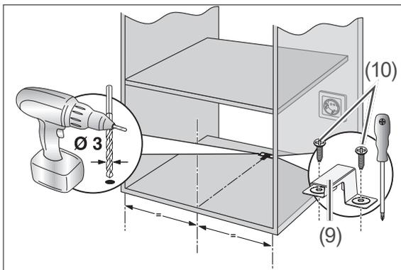
4. Drill holes (you need a 3-mm drill); reposition the anti-tip feature and screw it in with 2 screws (10) using a cross-headed screwdriver.
