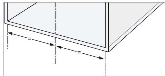
1. Determine the centre of the width of the built-in cupboard by measuring.
