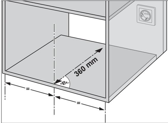
2. Draw an auxiliary line of 360 mm in length at right angles to this.
