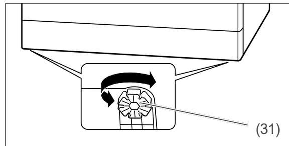
5. In order to compensate for uneven floor surfaces and set up the appliance horizontally, you can screw the four adjustable feet (31) in or out. The adjustable feet have slots around their circumference. Insert a screwdriver and turn the adjustable foot. Use a spirit level to set up the appliance.
