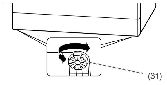
3. In order to compensate for uneven floor surfaces and set up the appliance horizontally, you can screw the four adjustable feet (31) in or out. The adjustable feet have slots around their circumference. Insert a screwdriver and turn the adjustable foot. Use a spirit level to set up the appliance.
