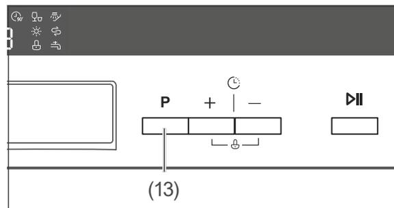
2. Press and hold the **P** button (13) for as long as required until the current water hardness is shown on the display: H 1 to H 5.
