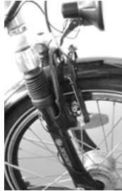
Suspension forks with elastomer/spring damping
