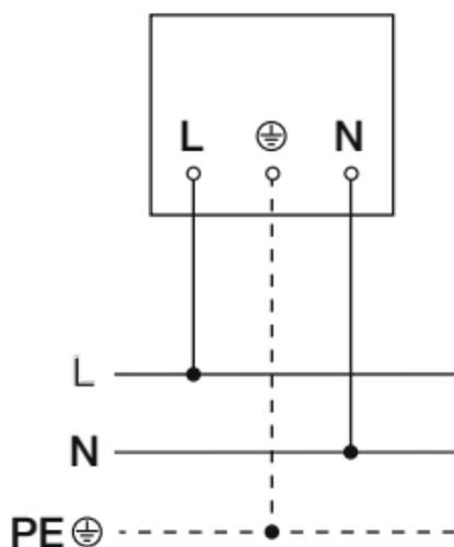
The mains power supply lead is a 3-core cable:
