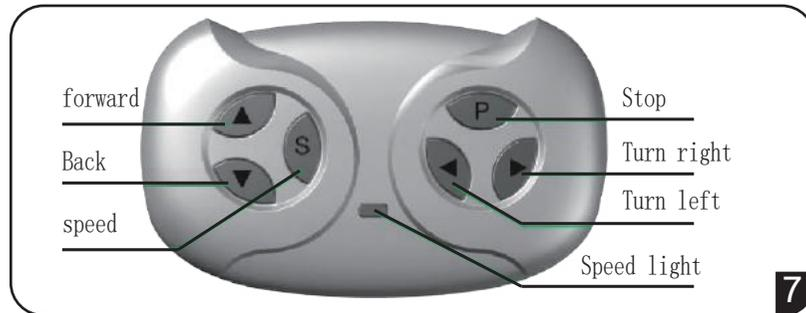
1. Press two buttons of “forward” and “backward” about 3 seconds to start the code and the light is glittering.
