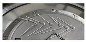
Step 2: 1) Take the CLOCK BOARD out from frame then turn around to the front, unscrew the GOLD NUT (in CCW) by a pair of pliers, then we can take off the hands.
