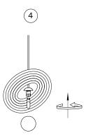
Apply the bulb & glass by rotating
