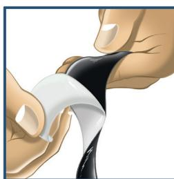
2. Remove the protective film from the upper side of the tape and place the tape on the element to be repaired.
