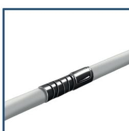
5. For the final winding, pull the tape less tightly and make sure that it overlaps completely. Press down the tape for 10 seconds until it is fixed in place.
