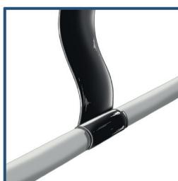
3. Apply the tape and hold it in place with your thumb. Pull the tape tight and wrap it around one time while it overlaps completely. This results in the tape being fixed in position for further wrapping.
