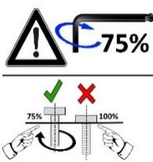
Please note that the screws are first inserted by hand and then only tightened slightly so that the screw is secure and the elements are loosely connected. Do not tighten the screws until all elements are connected in the correct way. Subsequent tightening of the screws can compensate for minor discrepancies in drill holes or weld points that can be present in hand-finished products.
