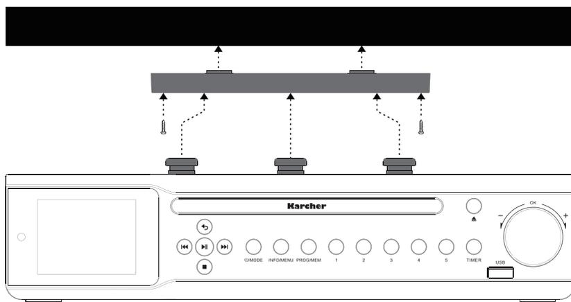
1. Remove the mounting plate from the unit by sliding it backwards.
