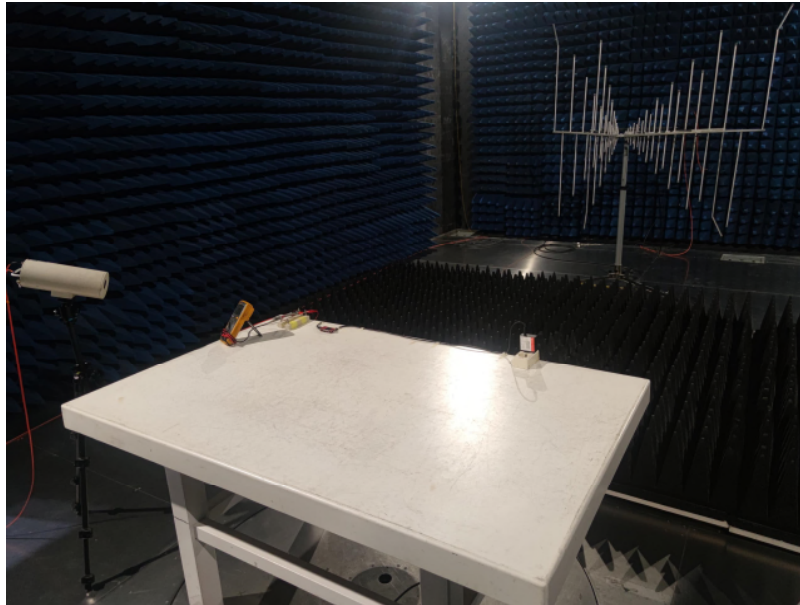
Photograph 5: Set-up for Radio-frequency Electromagnetic Fields (RS)
