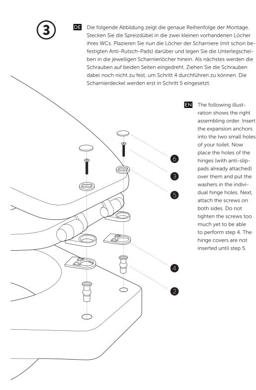
The following illustration shows the right assembling order. Insert the expansion anchors into the two small holes of your toilet. Now place the holes of the hinges (with anti-slippads already attached) over them and put the washers in the individual hinge holes. Next, attach the screws on both sides. Do not tighten the screws too much yet to be able to perform step 4. The hinge covers are not inserted until step 5.
