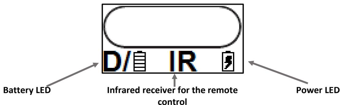
2. The status LED indicates the current battery status during the charging process.
