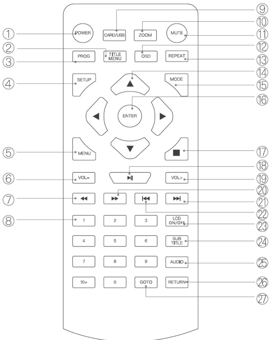
The remote control uses infrared waves (IR). Hold the remote control in the direction of the TV set. If the remote control is out of range or angle, the remote control may not work properly. To avoid battery leakage, remove the batteries from the remote control if the device is not to be used for a longer period of time.
