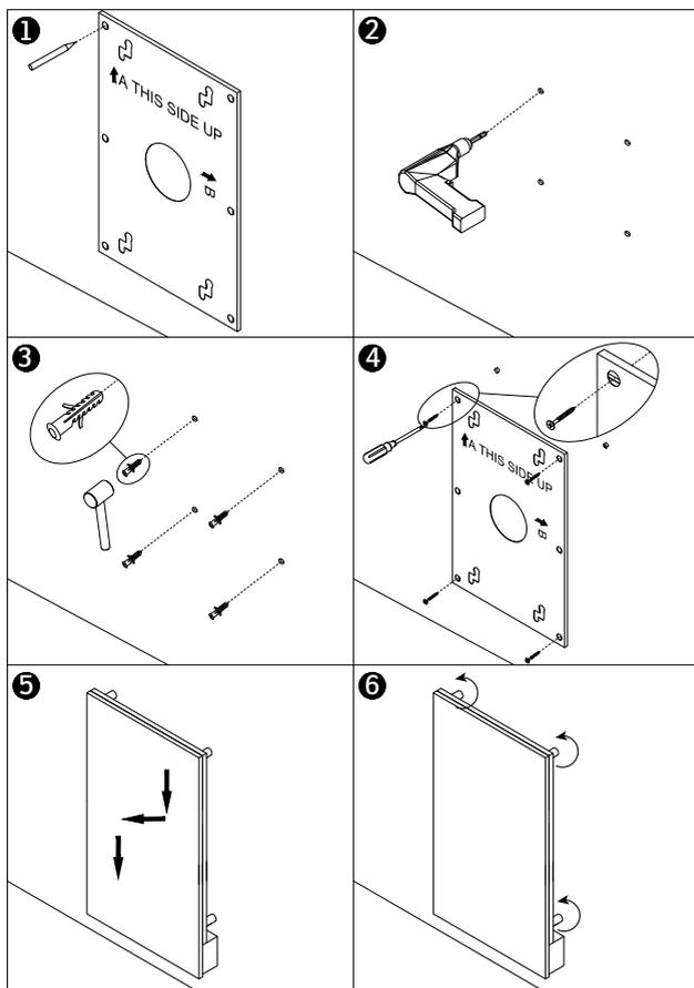
1. mark the position of the holes on the wall using the template provided
