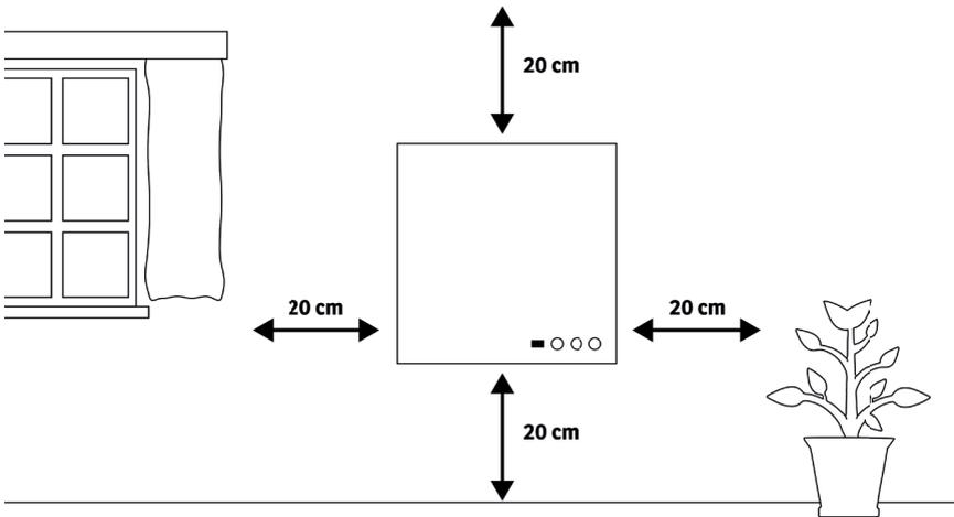
The heater must be at least 20 cm away from all objects, walls, the ceiling and the floor.
